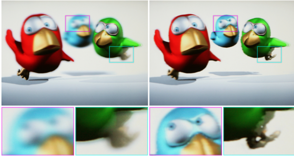
Figure 1: Applying perceptual considerations to improve the viewing experience (for the case of multiview and stereo content). Left: a computational model of human perception allows to overcome display-specific depth of field limitations for automultiscopic displays; details in blurred areas are recovered, while maintaining the apparent depth of the displayed objects [Masia et al. 2013a]. Right: a novel metric of visual comfort for stereo motion predicts comfort zones as a function of velocity, disparity and spatial frequency of the luminance; regions outside those zones should be avoided when creating stereo content [Du et al. 2013].
